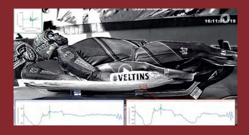
With Motion Amplification® software an ROI (region of interest) can be drawn anywhere in the image to extract vibration frequency and amplitude data.
