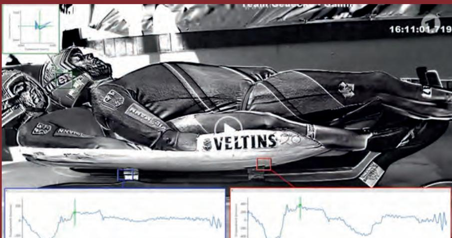
With Motion Amplification® software an ROI (region of interest) can be drawn anywhere in the image to extract vibration frequency and amplitude data.
