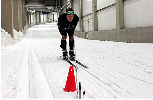
Abb. 1: Gliding test in ski tunnel. The start and endpoint reflector and the optical sensor on the right calf of the tester can be seen.
