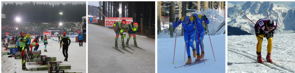
Fig. 3: Ski technician with prepared skis in the stadium area. b) Pair tests to determine differences in the glide behaviour of the individual skis. c) Change of the skis. d) Glide test on a defined course.
