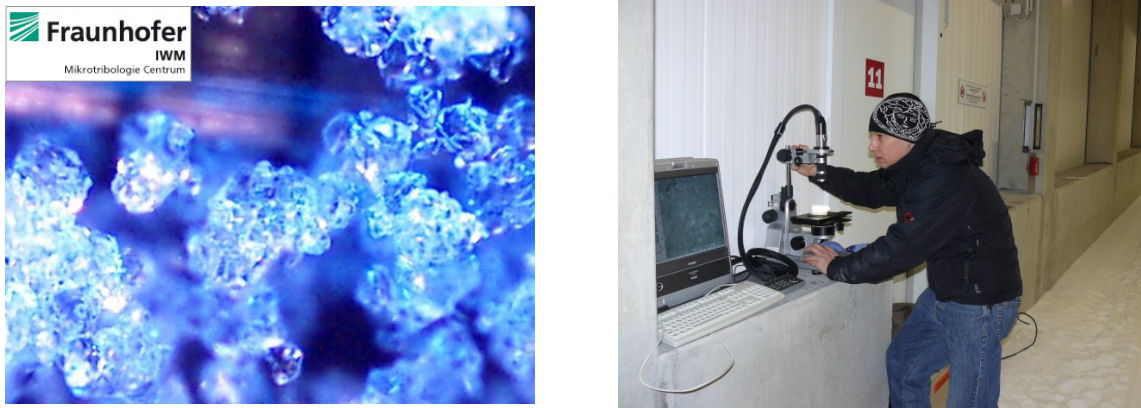
Fig. 1: Competition snow, Oberhof 2009, Kulle curve. Snow microscopy in the Oberhof ski tunnel.
