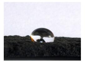
Figure 47: A drop of water on a surface of alkane bonded E-indigo.
