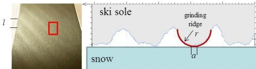
**Figure 2:** Left: Photography of grinding ridges. Right: Schematic of the grinding structure with single ridges contacting snow. The length  $l$  has to be chosen carefully in order to reflect the grinding structure of the ski.
