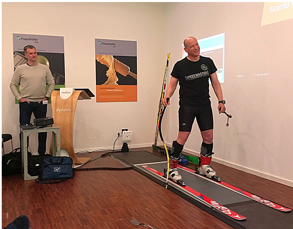
Figure 3: Pressure distribution measurements performed by Dr. Jens Hollenbacher using a molibso hi-res plate.
